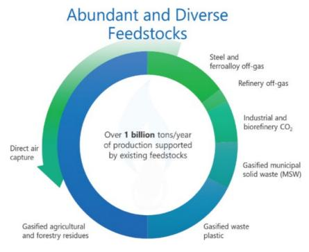
CO can provide both carbon and energy for our proprietary microbes. In contrast,  $CO_2$  only provides carbon, which means a source of chemical energy,  $H_2$ , must be added for a  $CO_2$  conversion. In a CO-rich stream, the microbe can make the  $H_2$  it needs from water via a biological water gas shift reaction, creating CO waste streams of various compositions ideal for gas fermentation.
