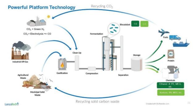
**Step 1:** The process begins by receiving off-gas or waste gas streams comprising gases that contain various mixtures of CO, CO<sub>2</sub> and H<sub>2</sub>, such as from steelmaking emissions or gasified waste.
