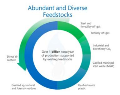
CO can provide both carbon and energy for our proprietary microbes. In contrast,  $CO_2$  only provides carbon, which means a source of chemical energy,  $H_2$ , must be added for a  $CO_2$  conversion. In a CO-rich stream, the microbe can make the  $H_2$  it needs from water via a biological water gas shift reaction, creating CO waste streams of various compositions ideal for gas fermentation.
