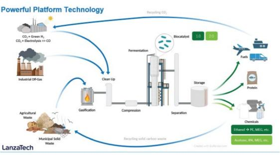
**Step 1:** The process begins by receiving off-gas or waste gas streams comprising gases that contain various mixtures of CO, CO<sub>2</sub> and H<sub>2</sub>, such as from steelmaking emissions or gasified waste.
