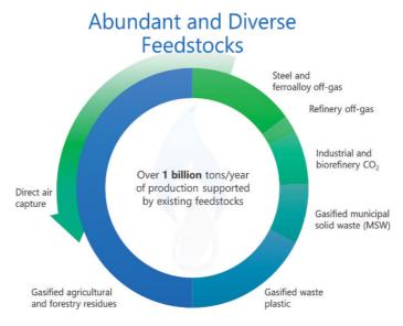
CO can provide both carbon and energy for our proprietary microbes. In contrast, CO<sub>2</sub> only provides carbon, which means a source of chemical energy, H<sub>2</sub>, must be added for a CO<sub>2</sub> conversion. In a CO-rich stream, the microbe can make the H<sub>2</sub> it needs from water via a biological water gas shift reaction, creating CO waste streams of various compositions ideal for gas fermentation.
