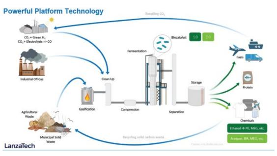
**Step 1:** The process begins by receiving off-gas or waste gas streams comprising gases that contain various mixtures of CO,  $CO_2$  and  $H_2$ , such as from steelmaking emissions or gasified waste.
