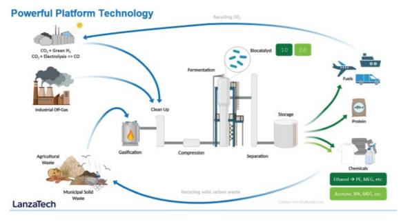
**Step 1:** The process begins by receiving off-gas or waste gas streams comprising gases that contain various mixtures of CO,  $CO_2$  and  $H_2$ , such as from steelmaking emissions or gasified waste.
