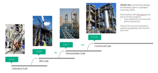
LanzaTech's gas fermentation process has been demonstrated at four sites with 50,000 hours of operation in the field using steel mill waste gases plus another 50,000 hours of operating in the field integrating gasification, gas treatment and gas fermentation. The success of these 100,000 hours of experience at pilot and demonstration scales
